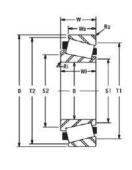
Tapered roller bearings are comprised of solid inner and outer rings with raceways, taper rollers and cages manufactured from pressed steel. The bearings are not self-retaining. As a result, the inner ring with the rollers can be fitted separately from the outer ring. Tapered roller bearings are not sealed and not supplied grease filled.
